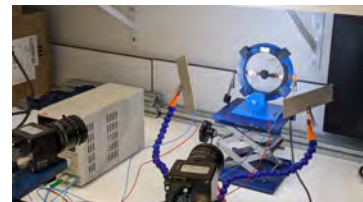
Experimental setup used to observe the displacements produced by the DEA prototype when tension is applied.
